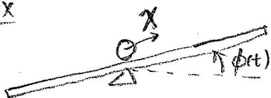
$$m\ddot{x} = mg \sin \phi(t) \quad \text{Nonlinear model.}$$
